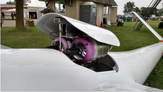
After reaching altitude, the engines are shut down and allowed to cool. Once cooled, both engines are retracted back into the fuselage to reduce drag.
